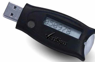
Figure 2: Secure Token Capable of OTP and PKI Authentication
